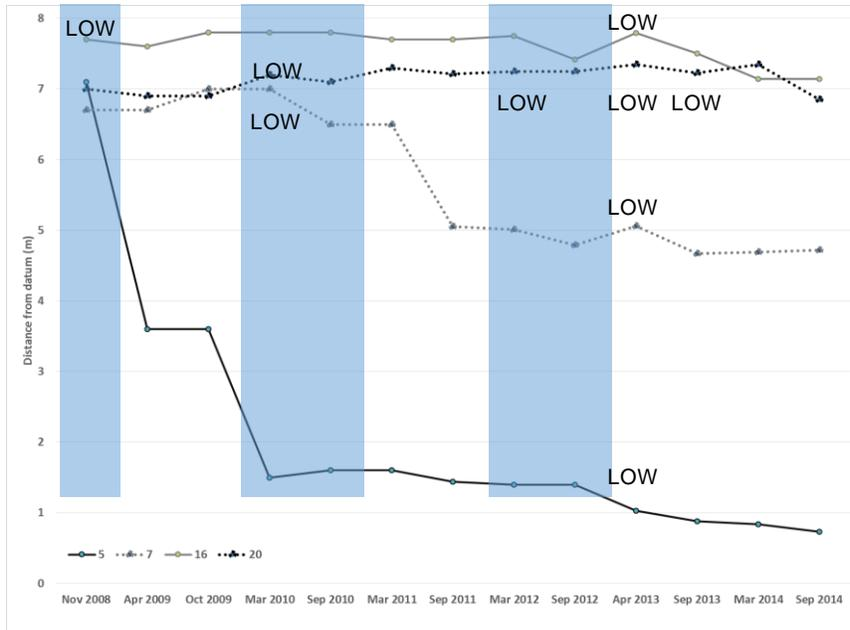
Figure 9. Cliff recession data (distance to cliff edge) measured in Filey Bay. Wet years are highlighted by shaded zones. Periods of lower than average beaches are marked “LOW”.
