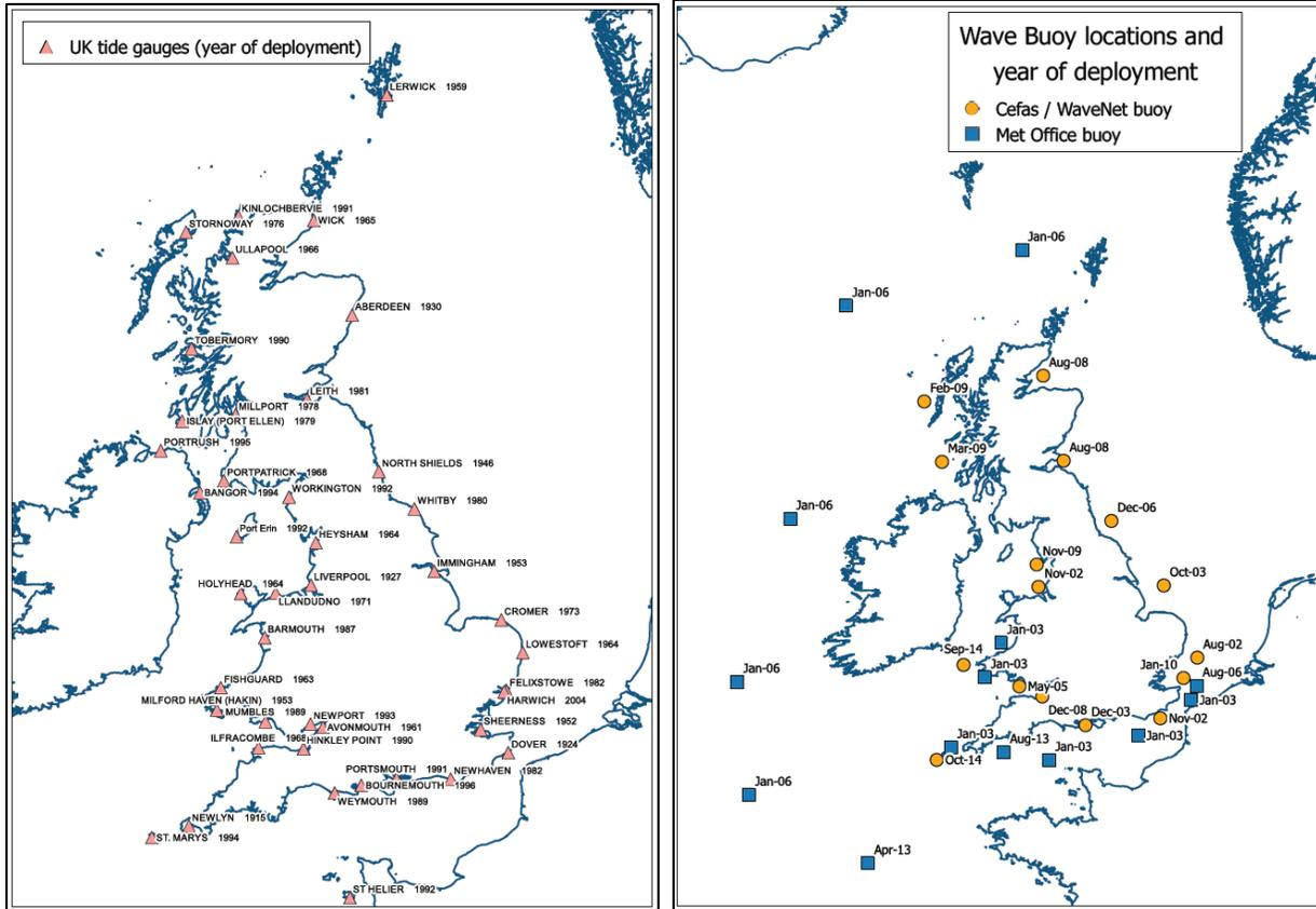
Figure 2 Location of the UKCMF tide gauges and WaveNet wave buoys showing deployment year for each site
