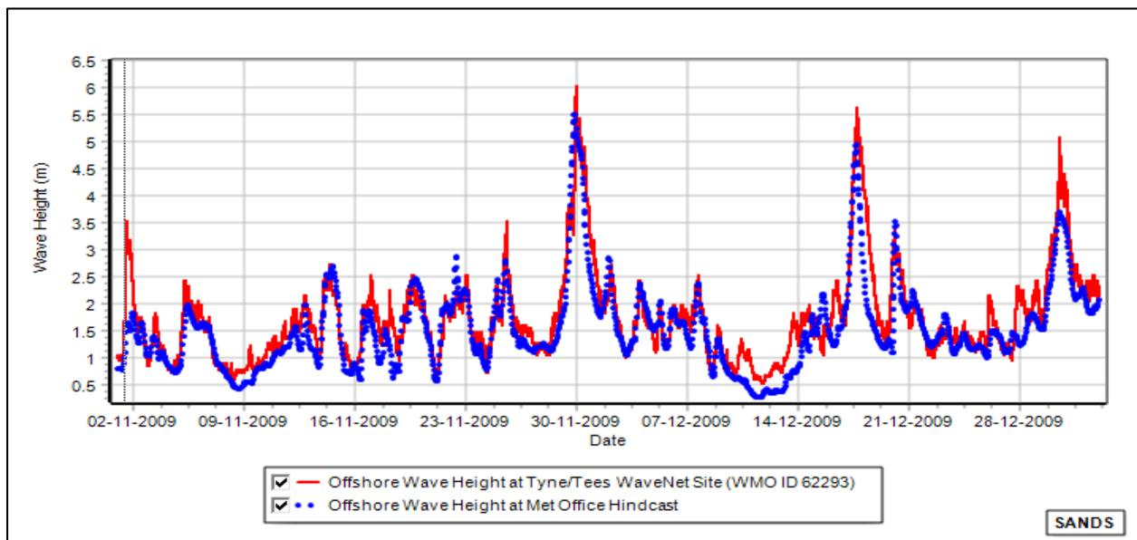
Figure 7 Example plot of hindcast and measured wave data at Tyne Tees in winter 2009
