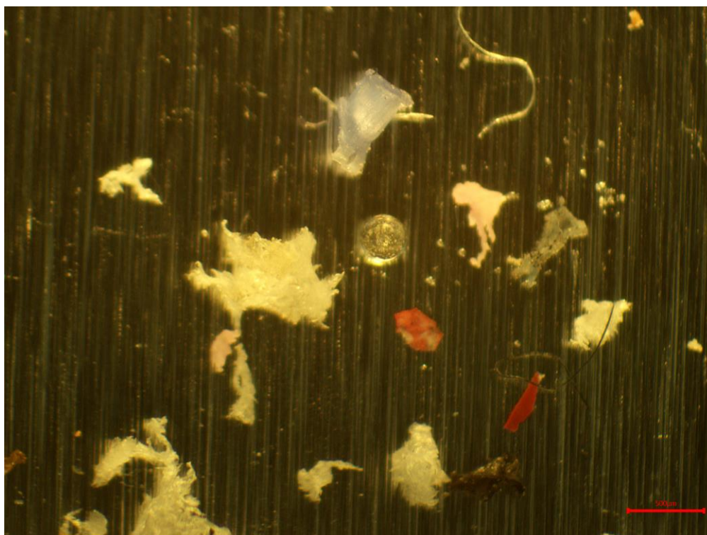
Figure 1. Overview image of potential microplastics recovered from sample ASC36266.001 (A1 1)
