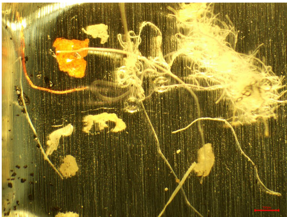
Figure 12. Overview image of potential microplastics recovered from sample ASC36266.012 (C4 1)
