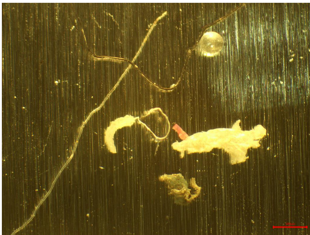
Figure 20. Overview image of potential microplastics recovered from sample ASC36266.020 (E2 1)
