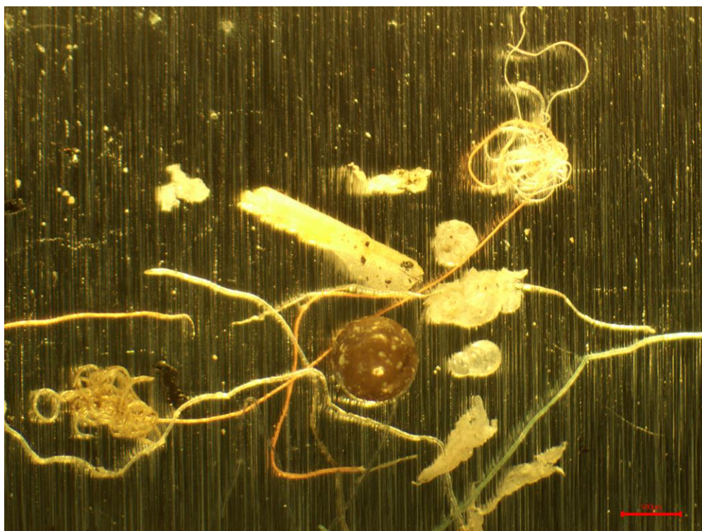
Figure 16. Overview image of potential microplastics recovered from sample ASC36266.016 (D2 2)
