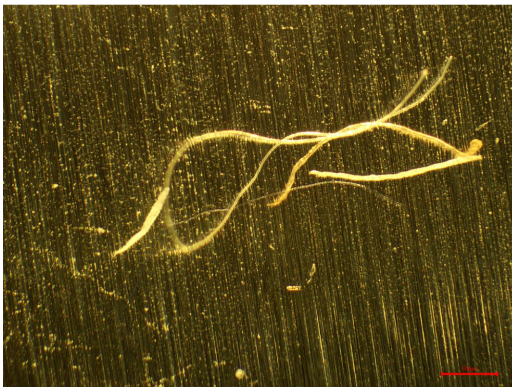
Figure 15. Overview image of potential microplastics recovered from sample ASC36266.015 (D2 1)
