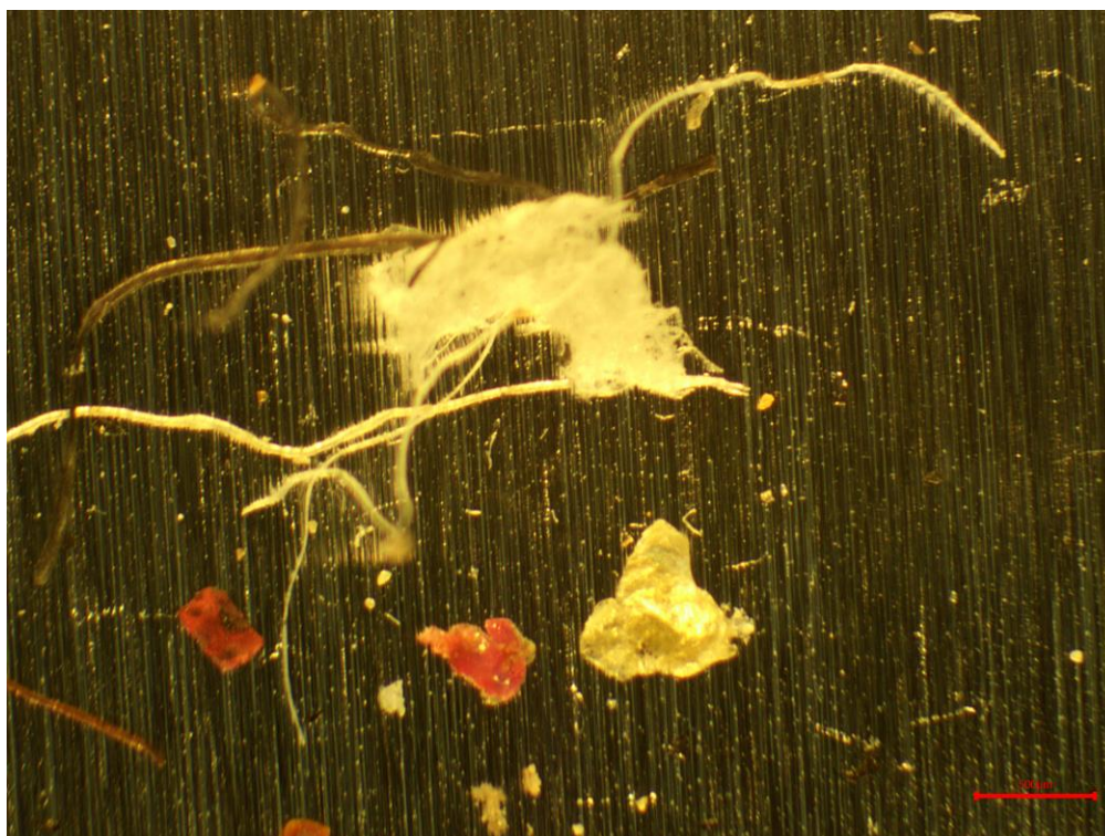
Figure 6. Overview image of potential microplastics recovered from sample ASC36266.006 (B2 2)
