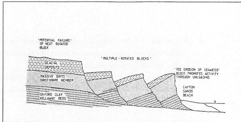
Figure 4.2 Section through Tenant's Cliff landslide complex
