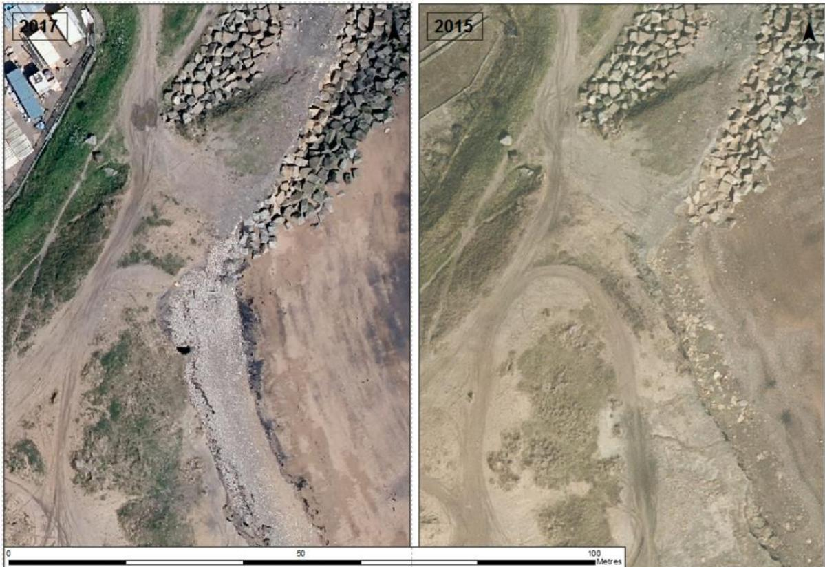
Figure 3 – Coastal erosion at the southern end of the Lynemouth rock revetment
